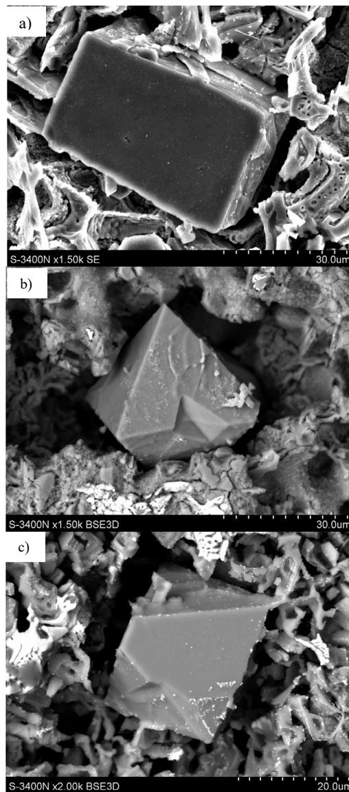
Fig. 4. Microstructure of the AlSi17 alloy: a) without overheating; b) after overheating to 840°C; c-f) after overheating to 920°C; a-c) LM; d-f) SEM; e-f) deeply etched sections
