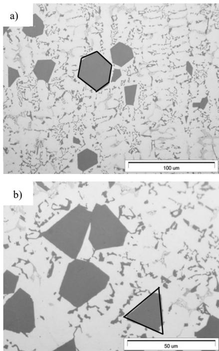
Fig. 6. Microstructure of the AlSi17 alloy after overheating to approximately 920°C with the cross-sectional plane of primary silicon crystals in the shape of: a) hexagon; b) triangle
