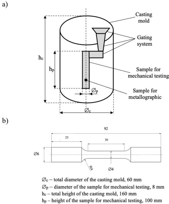
Fig. 2. Casting mould: a) diagram; b) dimensions of the sample for mechanical testing (mm)
