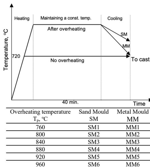
Fig. 1. Diagram and research plan of the overheating process of the AlSi17 alloy
