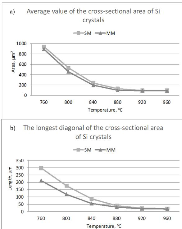
Fig. 7. Influence of overheating temperature on: a) surface area; b) the longest diagonal of the cross-section of primary silicon crystals (average values)
