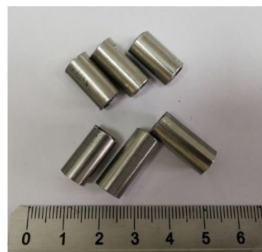
Fig. 1. SS316 samples prepared for testing
