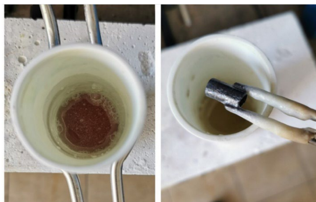
Fig. 2. Crucible with molten salt (left) and the SS316 steel sample immediately after being removed from the molten salts
