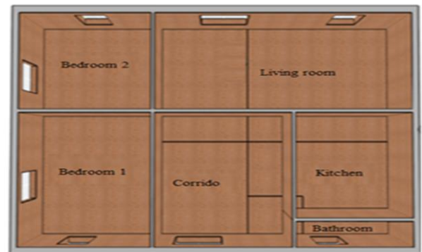
Fig. 2. Layout of zones on the first floor. This model was created with DesignBuilder software.
