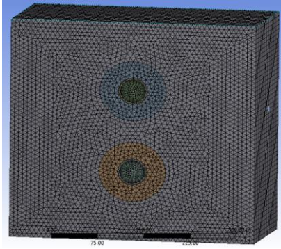
Fig. 7. The geometry model after discretization process (mapped mesh type applied: prism).
