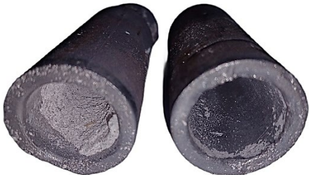
Fig. 8. Comparison of Castings: Traditional Mould (Left) vs. Weakened Mould (Right)
