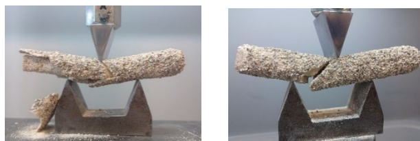
Fig. 4. Bending strength of ceramic moulds
