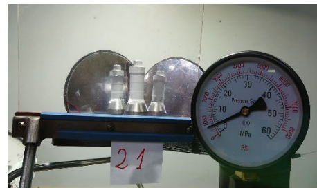
Fig. 20. System of mirrors for tracking surfaces of samples from three sides in real time
