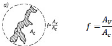
Fig. 8. Scheme of shapes of graphite precipitate cross-sections [8]
