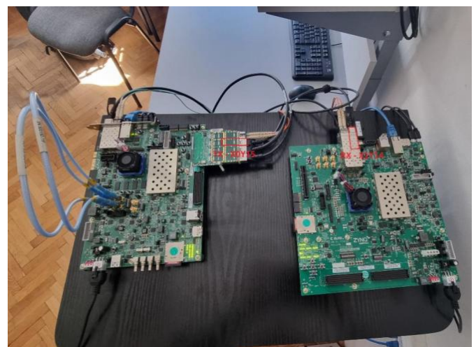
Fig. 10. Test setup. On the left is a ZCU106 board, serving as a transmitter, and on the right is a ZCU102 board, serving as a receiver. An additional SFP+ FPGA Mezzanine Card was used for testing loop-back mode with different clock signal generators
