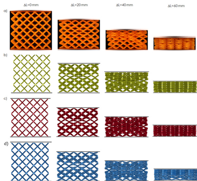
Fig. 16. Comparison of the BCC lattice structure deformation process: a) experimental tests and FEA with three different crosssections for the struts: b) hexagonal, c) round, and d) square
