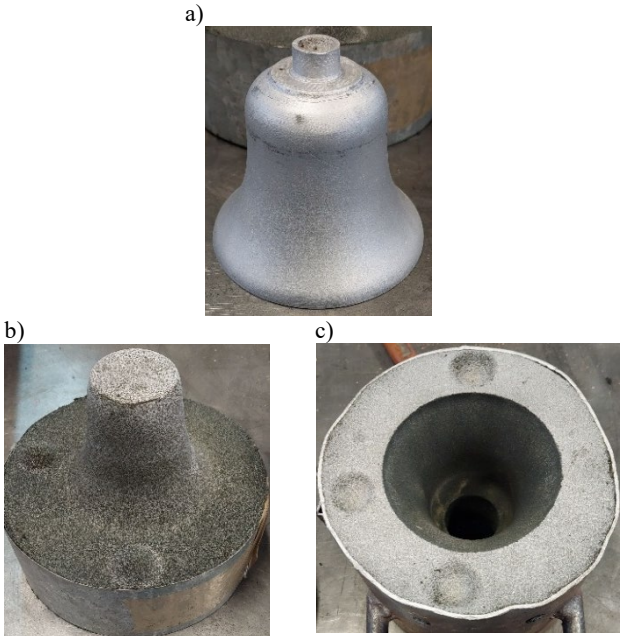
Fig. 5. 3D-printed pattern (a) and drag mold /core (b) and cope mold (c)
