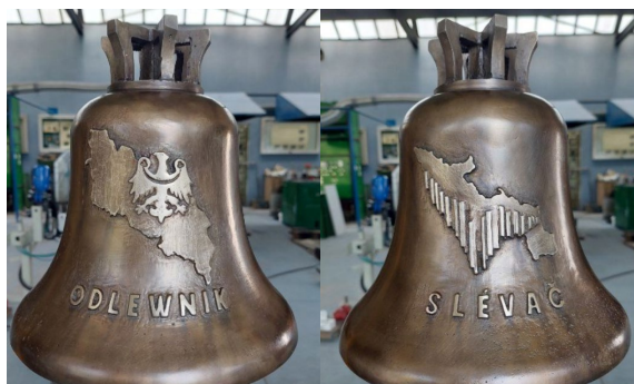
Fig. 6. Bell DZ2: cast from a mold made with a 3D-printed pattern (front and rear views)
