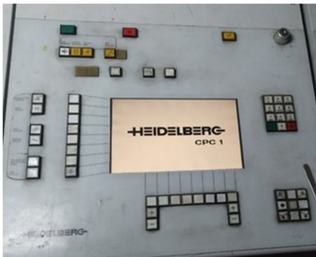
Fig. 4. CPC 1.04 control panel, the only IIoT gathering point for information analyses on SM74-4P 1997, source: own elaboration based on (Heidelberg, 1997)
