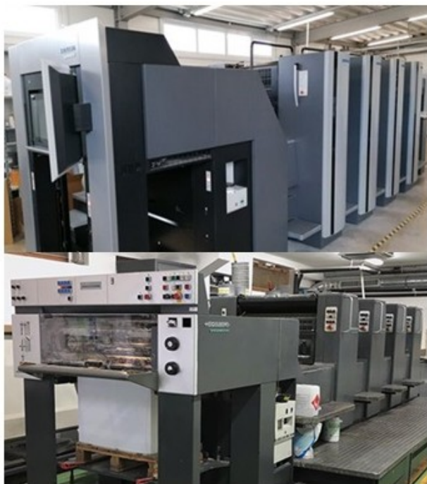
Fig. 7. Retrofitted Heidelberg Speedmaster SM74-4 from 1997 (below) and newest CX75-4 Heidelberg model as from 2021 (above), source: own elaboration
