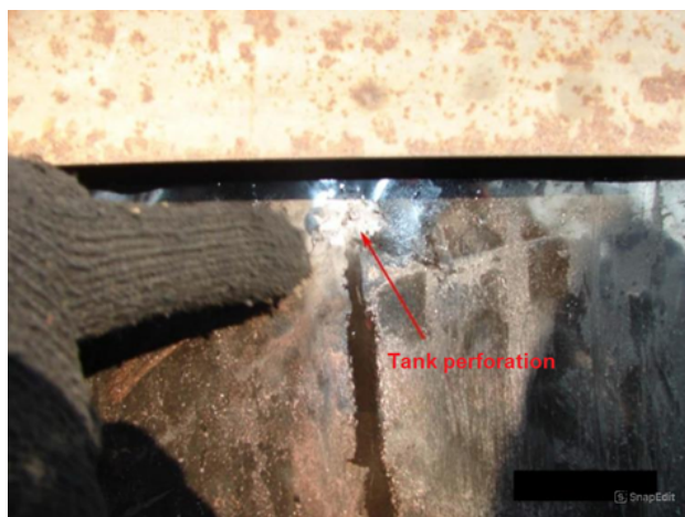
Fig. 11. Fuel tank shot through with .308 WIN Match bullet – shot 20, with characteristic leakage of tank contents
