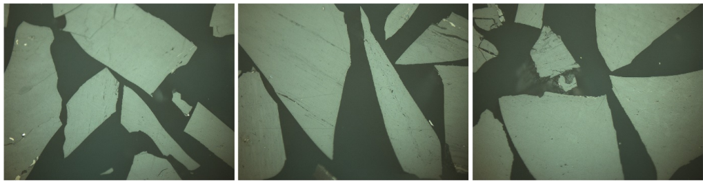
Fig. 3. Microscope images of N1 fraction (predominantly composed of vitrinite macerals, mainly collotelinite), oil immersion, magnification 500×
