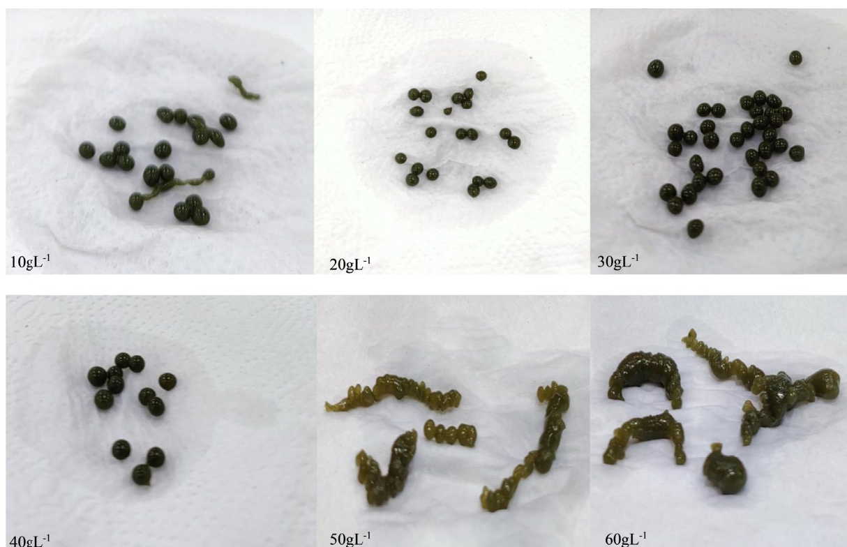
Fig. 3. Shape of alginate beads from different alginate concentrations
