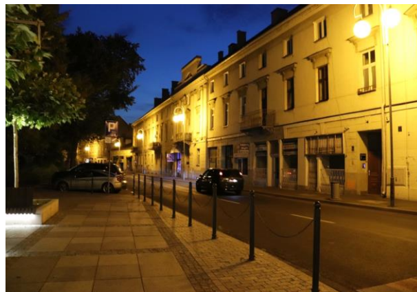
Fig. 3. Lighting of Babina Str. in Kalisz (Poland) implemented using spherical luminaires with a high ULOR coefficient [Photo: Author, 14.07.2023].
