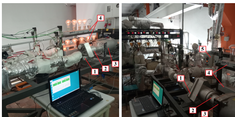
Figure 1. Test rig for the expansion microunit: 1 – scroll expander, 2 – clutch, 3 – generator, 4 – generator load system, 5 – heat source.
