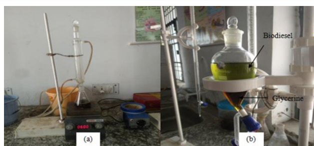
Fig. 3. Biodiesel preparation: (a) magnetic stirring, (b) biodiesel and glycerine separation.
