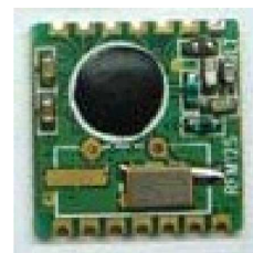
Fig. 11. View of universal ISM band FSK module RFM12B used for signal transfer between stationary and mobile part of the CET system
