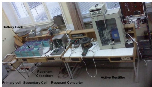
Fig. 13. View of the laboratory setup with 15kW bi-directional CET system
