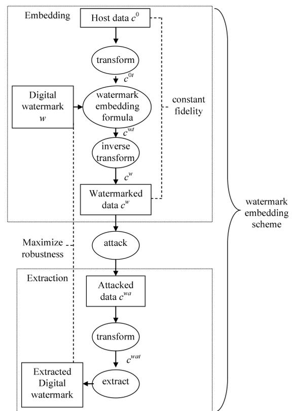
Fig. 1. Scheme of transform-based digital watermarking
