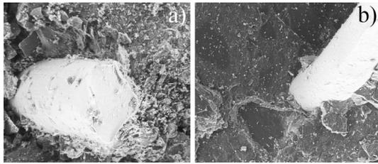
Fig. 14. Steel fibre in RPC, (a) curing in water, (b) autoclaving, magnification 500x
