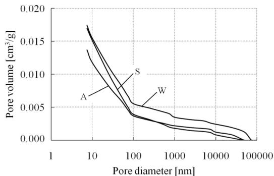
Fig. 16. Effect of different curing conditions on RPC microporosity
