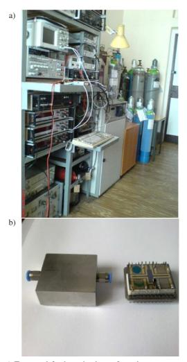
Fig. 6. a) Test-stand for investigations of graphene structures in an atmosphere of synthetic air with the tested gas; b) gas chamber containing the resistance sensor structure
