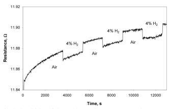
Fig. 8. Sensitivity of the graphene sensor structure to the presence of hydrogen in synthetic air (temperature of the structure 50°C, humidity of the air RH about 5%)
