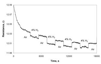
Fig. 9. Sensitivity of the graphene sensor structure to the presence of hydrogen in synthetic air (temperature of the structure 120°C, humidity of the air RH about 5%)
