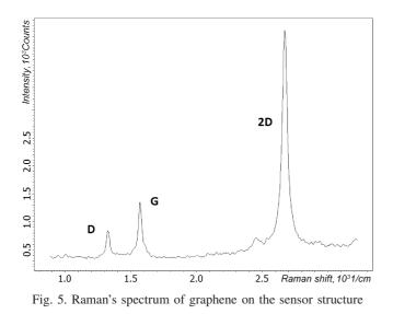
Three Raman peaks of graphene are visible in this spectrogram, viz. D, 2D, and G; Raman's spectrum confirms the fact that the layer deposited on the surface of the resistance transducer is a layer of graphene displaying favorable morphological properties.
