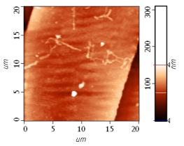
Fig. 20. AFM phase image of the surface of the electrode structure with graphene after numerous cycles of deposition of the synthetic air with NO<sub>2</sub> and steam
