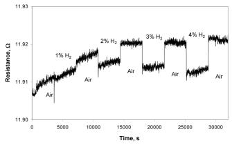
Fig. 10. Sensitivity of the graphene sensor structure to the presence of hydrogen in synthetic air (temperature of the structure 120°C, humidity of the air RH about 5%)
