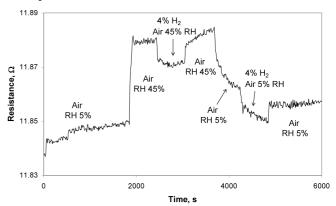
Fig. 15. The influence of humidity and the effect of hydrogen on the value of the resistance of a graphene sensor structure with a 3nm palladium layer (temperature of the structure 50  $^{\circ}$ C)
