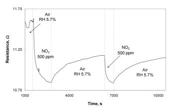
Fig. 17. Sensitivity of the sensor structure with graphene to the presence of NO<sub>2</sub> in the atmosphere of synthetic air (temperature of the structure 120°C, humidity RH about 5%)
