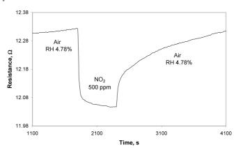
Fig. 18. Sensitivity of the sensor structure with graphene modified by a 3 nm Pd layer to the presence of NO<sub>2</sub> in the atmosphere of synthetic air (temperature of the structure  $120^{\circ}$ C, humidity RH about 5%)
