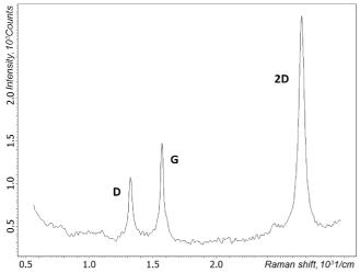
Fig. 19. Raman's spectrum of graphene on the sensor structure after its using in complex investigations
