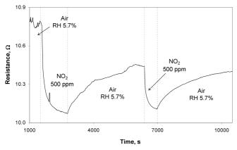
Fig. 16. Sensitivity of the sensor structure with graphene to the presence of NO<sub>2</sub> in the atmosphere of synthetic air (temperature of the structure  $50^{\circ}$ C, humidity RH about 5%)
