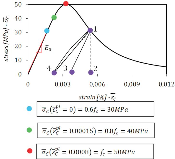
Fig. 11. Stress-strain dependence for compression of concrete damage plasticity model.
