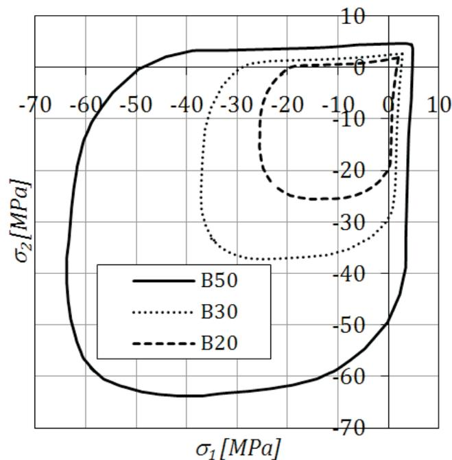
Fig. 1. Kupfer's curves for different class of concrete.
