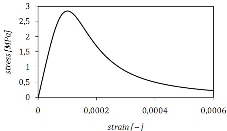
Fig. 8. Uniaxial compression of concrete [26].
