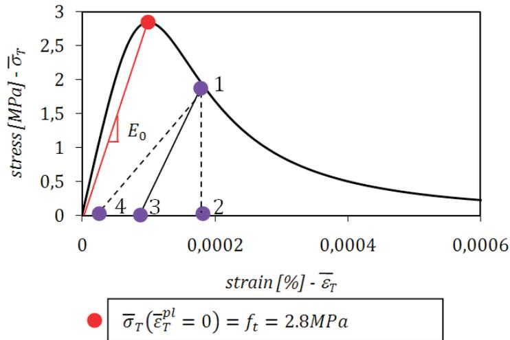
Fig. 12. The stress-strain dependence for tension of concrete damage plasticity model.
