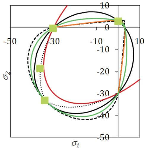
Fig. 3. Different failure criteria in plane stress conditions  $\sigma_1 - \sigma_2$ .
