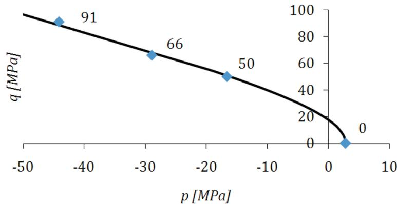
Fig. 15. Plastic flow potential function with identification points.
