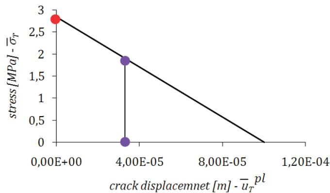
Fig. 13. Linear softening in tension.
