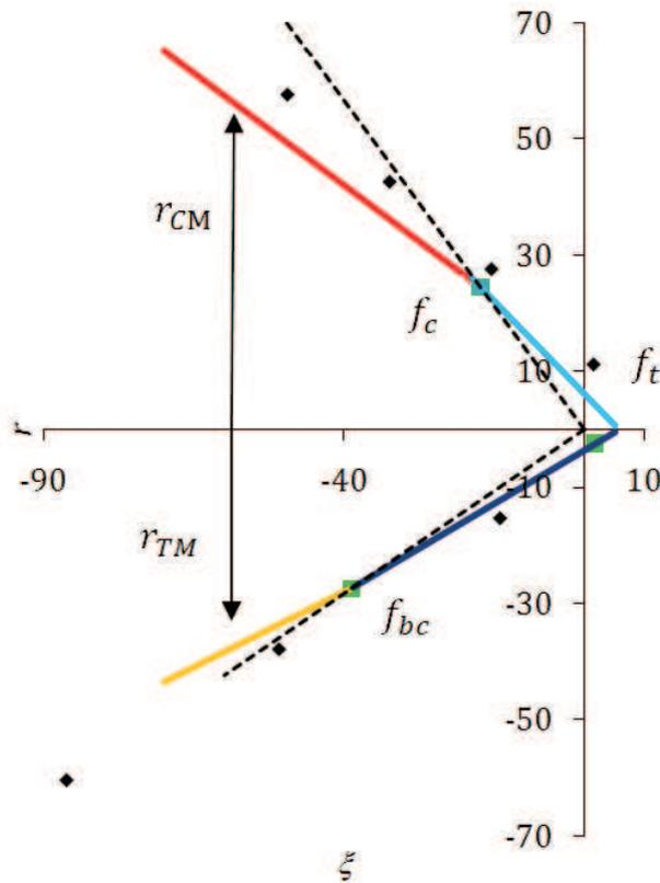
Fig. 6. Meridian plane of Lubliner loading function.
