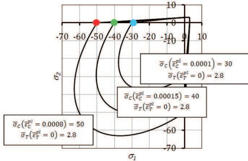
Fig. 14. Evolution of loading function in plane stress conditions.
