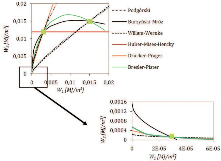
Fig. 2. Comparison of failure curves in space  $W_1 - W_2$ .
