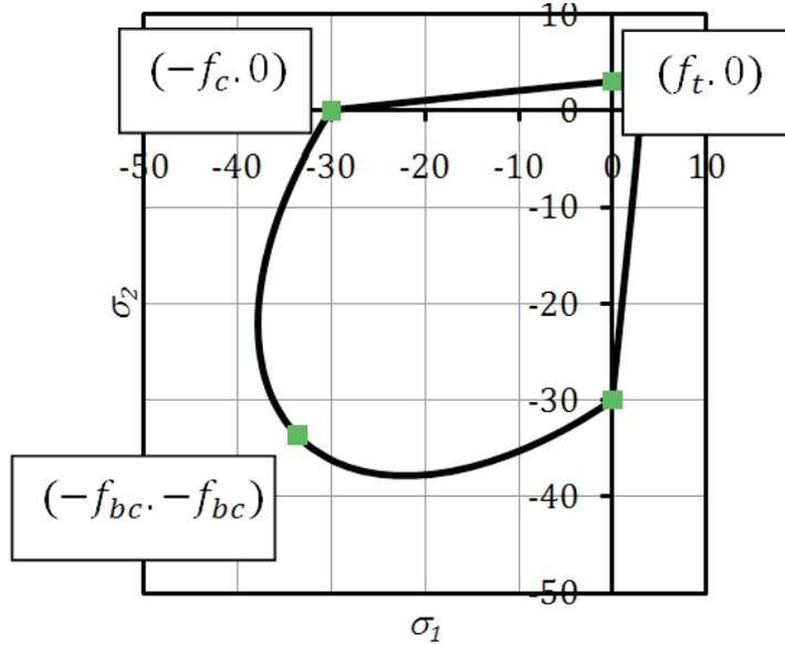
Fig. 5. Lubliner loading function in plane stress conditions.
