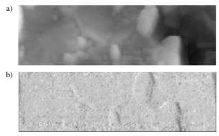
Fig. 7. Topography of graphene observed in tapping-mode made by dedicated software (a) and image of the second harmonic component (b)
