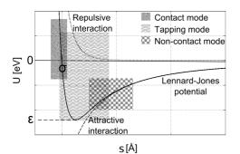
Fig. 3. Sketch of a typical tip-sample potential
