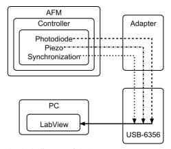
Fig. 5. Block diagram of the AFM measurement system
