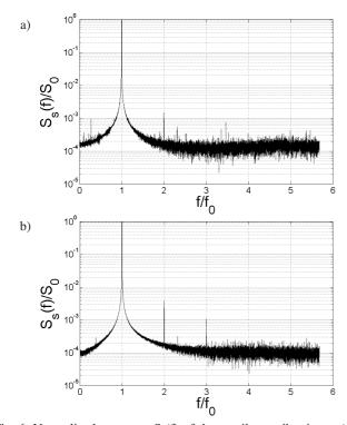
Fig. 6. Normalized spectrum  $S_s(f)$  of the cantilever vibrations: a) in air, b) in non-contact mode at vicinity of exemplary sapphire structure
