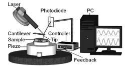
Fig. 2. The schematic setup of AFM
