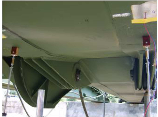
Fig. 3. A view of the location of potentiometric indicators used for displacements measuring
