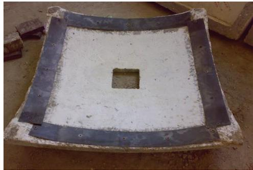
Fig. 8. Repaired shell by using steel strip.
