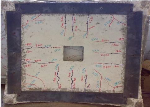
Fig. 23. Crack pattern of repaired by steel plate.
