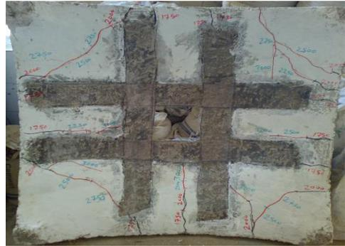
Fig. 24. Crack pattern of shell repaired by using 2 layers of GFRP (Type 1).
