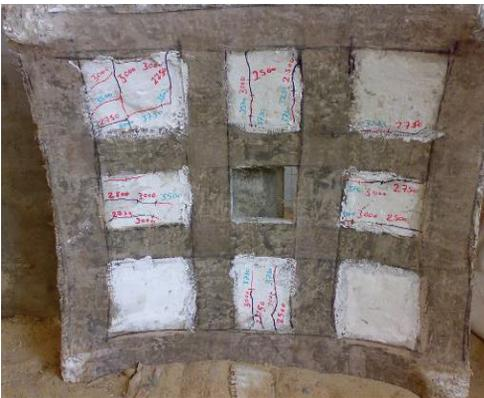
Fig. 25. Crack pattern of shell repaired by using 2 layers GFRP (Type 2).
