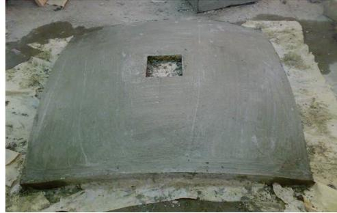
Fig. 2. Shell with central opening.
