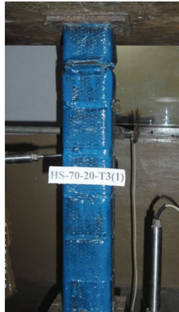
Fig. 12. Failure mode of column HS-70-20-T3(1)
