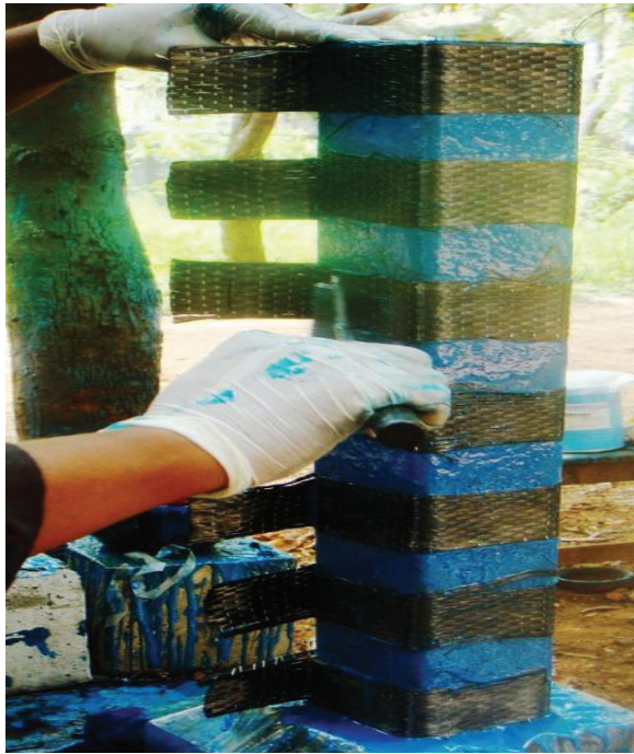
Fig. 4. Bonding of CFRP
