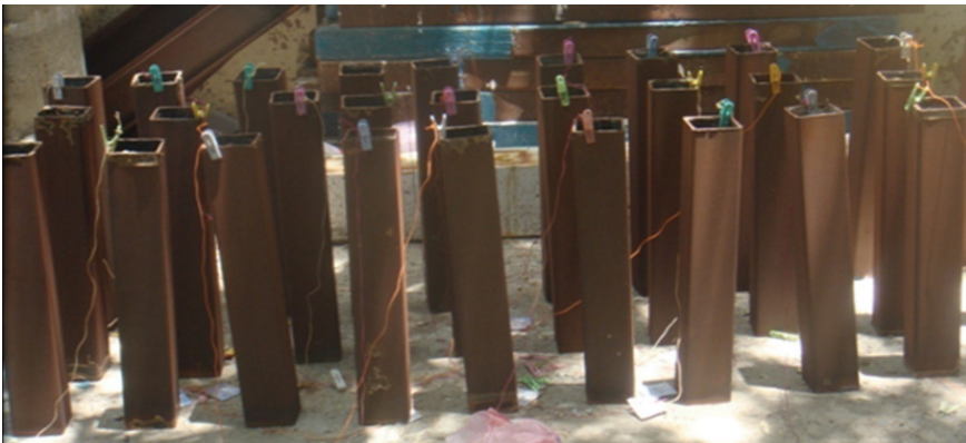
Fig. 3. Specimens after corrosion
