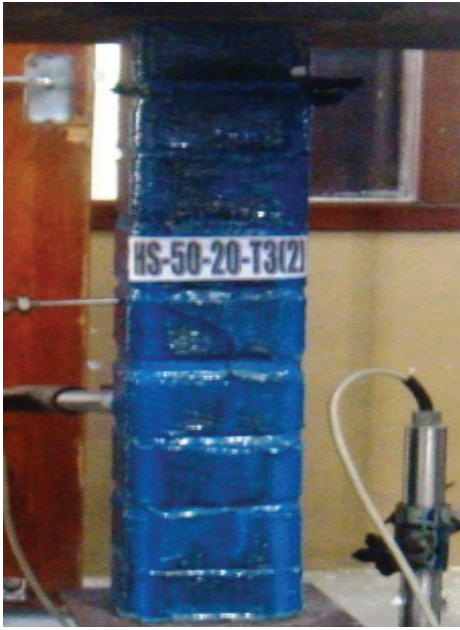
Fig. 9. Failure mode of column HS-50-20-T3(2)
