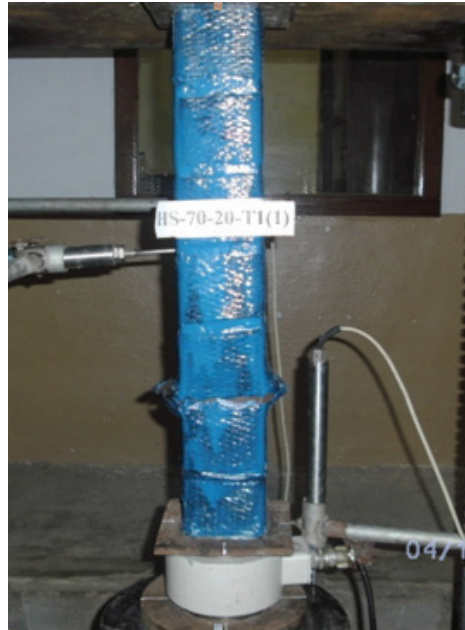
Fig. 10. Failure mode of column HS-70-20-T1(1)
