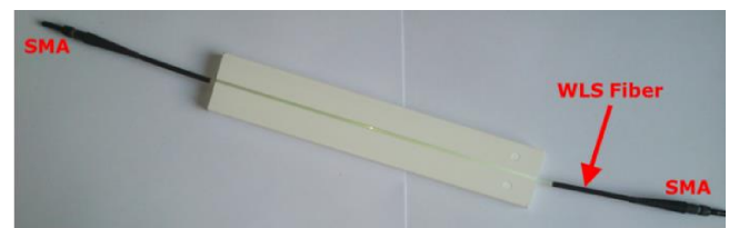
Fig. 4. WLS fiber placed in scintillator's groove
