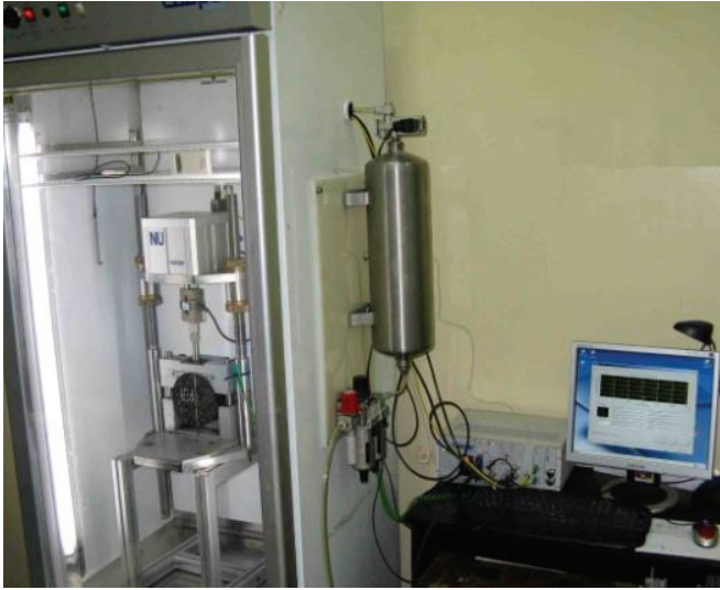
Fig. 3. Stand for fatigue tests using shearing
