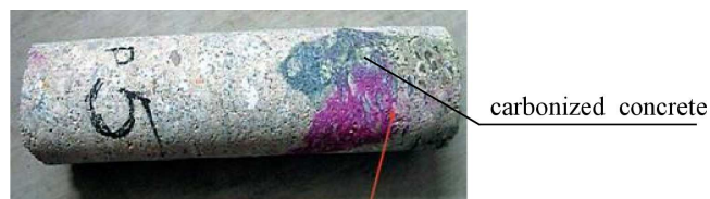
Fig. 17. Drilled core with carbonized concrete marked using rainbow test (Ref. 56)
