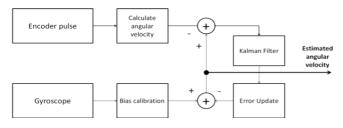
Fig. 4. Angular velocity composed of optical encoder and gyroscope
