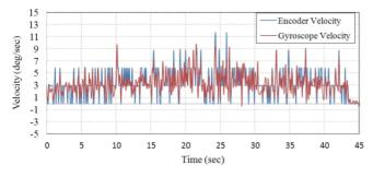
Fig. 3. The angular velocity measured dynamically
