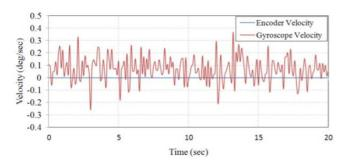
Fig. 2. The angular velocity measured statically
