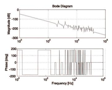
Figure 1. Bode plot of the free-free rotor, for  $\Omega = 0$  [rpm].
