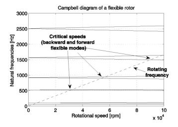
Figure 7. Campbell diagram of the flexible rotor in AMBs for  $\Omega$  from 0 to 100 000 [rpm].
