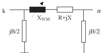
Figure 2. Equivalent model of TCSC.
