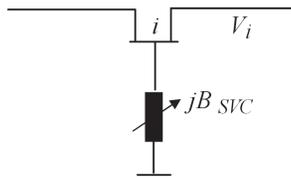
Figure 3. Equivalent model of SVC.
