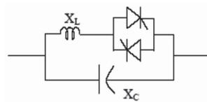
Figure 1. Structure of TCSC and SVC.
