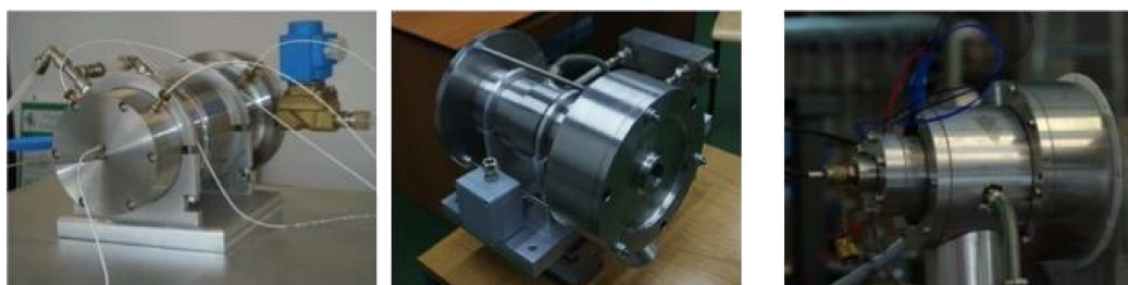
Fig. 3. Target design of Domestic Micro-CHP Unit with ORC after all examinations and tests in the laboratory of the IMP PAN in Gdansk, left – the first concepts, right – commercial version of the installation
