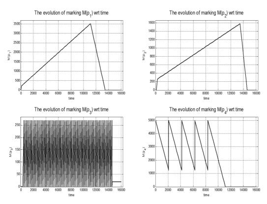
Figure 5. The dynamics behavior of the material flows of the production line in their individual scales - i.e. the marking evolution of the continuous places  $P_1 - P_4$  in time.
