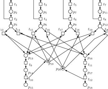
Figure 8. The Petri net-based model of the supervised cooperation of the production lines.
