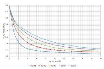
Fig. 3. PEVQ values as a function of packet losses and burst sizes at an encoding rate of 5175 kbps for the codec H.264/AVC and the MPEG-2-TS
