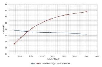
Fig. 5. Approximation of parameters P and Q as functions of the encoding rate for the codec  $\rm H.264/AVC$  and the MPEG-2-TS
