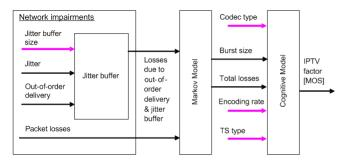
Fig. 1. Block diagram for the IPTV model
