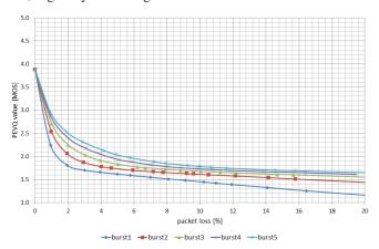
Fig. 2. PEVQ values as a function of packet losses and burst sizes at an encoding rate of 2125 kbps for the codec H.264/AVC and the MPEG-2-TS
