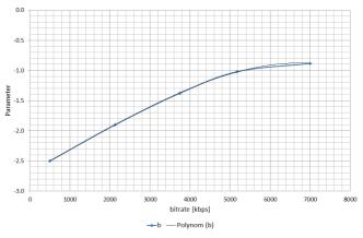
Fig. 7. Approximation of the parameter b as a function of the encoding rate for the codec H.264/AVC and the MPEG-2-TS
