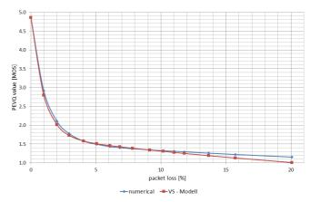
Fig. 11. QoS values as functions of packet losses gained from different measuring methods for the codec H.264/AVC and the MPEG-2-TS, a burst size of "1" and an encoding rate of 5175 kbps
