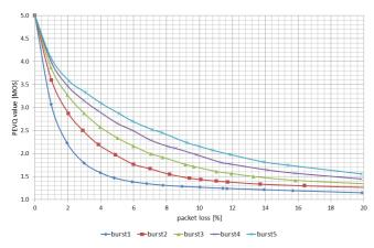
Fig. 4. PEVQ values as a function of packet losses and burst sizes at an encoding rate of 7000 kbps for the Codec H.264/AVC and the MPEG-2-TS
