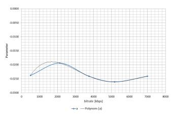
Fig. 6. Approximation of the parameter a as a function of the encoding rate for the Codec H.264/AVC and the MPEG-2-TS
