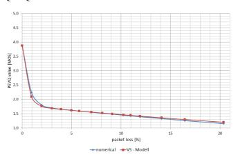
Fig. 9. QoS values as functions of packet losses gained from different measuring methods for the Codec H.264/AVC and the MPEG-2-TS, a burst size of "1" and an encoding rate of 2125 kbps
