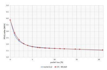
Fig. 10. QoS values as functions of packet losses gained from different measuring methods for then codec H.264/AVC and the MPEG-2-TS, a burst size of "3" and an encoding rate of 2125 kbps
