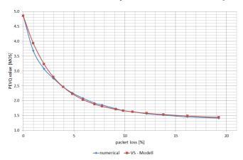
Fig. 12. QoS values as functions of packet losses gained from different measuring methods for the codec H.264/AVC and the MPEG-2-TS, a burst size of "3" and an encoding rate of 5175 kbps
