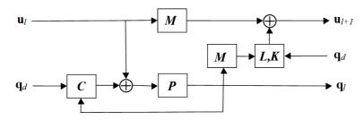
Figure 1. Learning control scheme with a feedback controller attached.
