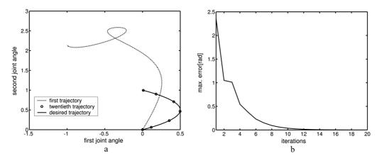
Figure 5. a) The initial, twentieth, and desired trajectory; b) Convergence of the maximal tracking error  $e_l^{\text{max}}$  for  $K_v = 0$ ,  $L_v = 0$  and  $K_p = 0$ ,  $L_p = 0$ .
