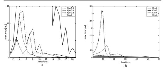
Figure 6. a) The profiles of maximal tracking error  $e_l^{\text{max}}$  for  $K_v = 0$ ,  $L_v = 0$ ; and  $K_p = 0.3$ , 0.6, 0.9, 2,  $L_p = 0$  b) The profiles of maximal tracking error for  $K_v = 1$ , 2, 4, 8,  $L_v = 0$  and  $K_p = 0$ ,  $L_p = 0$ .
