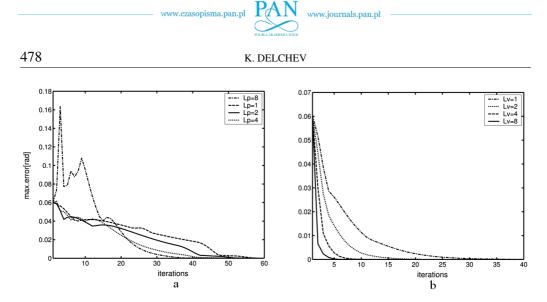
Figure 7. a) The profiles of maximal tracking error for  $K_v = 8$ ,  $L_v = 0$  and  $K_p = 1$ ,  $L_p = 1$ , 2, 4, 8; b) The profiles of maximal tracking error for  $K_v = 8$ ,  $L_v = 1$ , 2, 4, 8 and  $K_p = 1$ ,  $L_p = 2$ .
