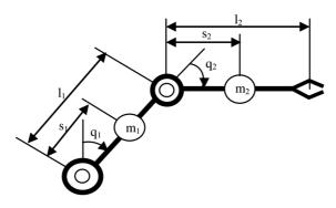
Figure 3. Kinematic scheme of SCARA-type horizontal robot arm.
