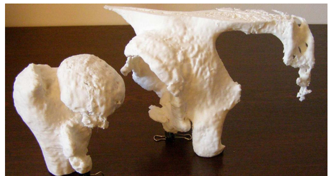
Fig. 7. Pelvic bones model made by MEM technique
