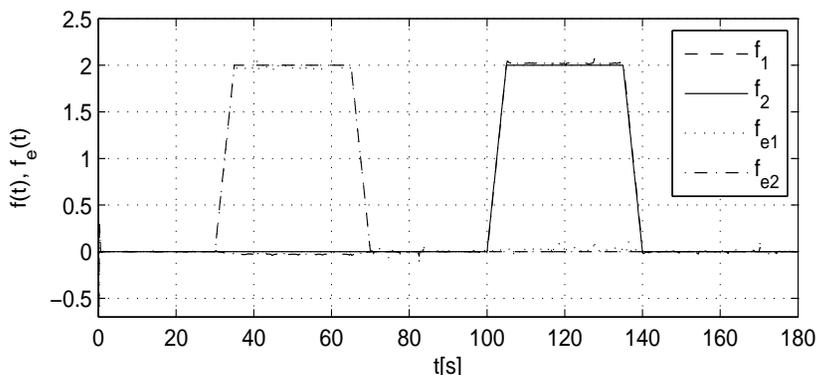
Figure 1: Single actuator faults and their estimates.
