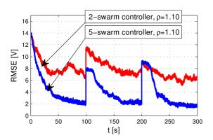
Fig. 8. Comparison of the RMSE graphs for the 2-swarm and 5-swarm controllers in the case of fast knowledge evaporation  $(\rho = 1.10)$
