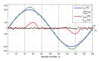
Fig. 9. The shape of the output voltage under the diode rectifier load for the 5-swarm controller – the load current, the commanded average voltage for the VSI and the control error added for clarity
