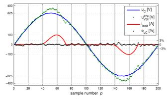
Fig. 12. The shape of the output voltage under the diode rectifier load for the 10-swarm controller and  $\rho = 1.20$  – the load current, the commanded average voltage for the VSI and the control error added for clarity
