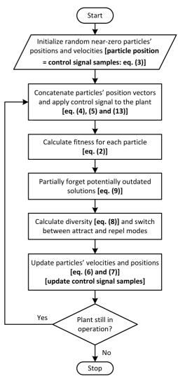
Fig. 5. A flowchart of the swarm repetitive controller
