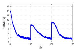
Fig. 15. Evolution of the RMSE for the "extreme" case of optimization space divided into 4D subspaces, i.e. 50-swarm controller, and  $\rho = 1.50$
