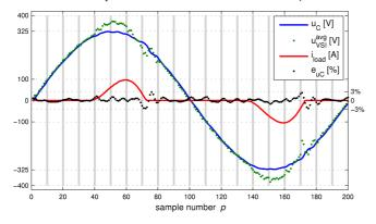
Fig. 14. The shape of the output voltage under the diode rectifier load for the 20-swarm controller and  $\rho = 1.40$  – the load current, the commanded average voltage for the VSI and the control error added for clarity
