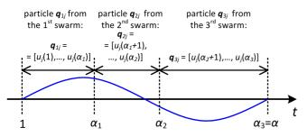
Fig. 2. The multi-swarm approach: a single particle from a subswarm covers only the subset of samples of the control signal related to the entire period of the depicted reference signal – the scenario with 3 swarms and a non-even task distribution
