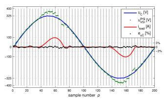
Fig. 16. The shape of the output voltage under the diode rectifier load for the 50-swarm controller and  $\rho = 1.50$  – the load current, the commanded average voltage for the VSI and the control error added for clarity
