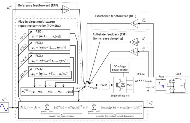
Fig. 4. A schematic diagram of the control system including a full-state feedback controller and a repetitive disturbance feedforward path – the exemplary nonlinear load depicted for clarity (the block labeled as Load)
