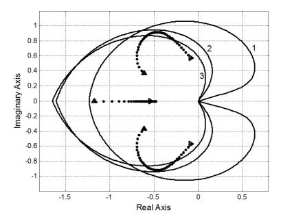
Figure 2: Eigenvalues of B (' $\triangleright$ '), C (' $\Delta$ '), the eigenvalue-loci of (3), (16) ('.') and stability regions for few values of  $\alpha$ :  $\alpha = 0.2$  (boundary 1);  $\alpha = 0.6$  (boundary 2) and  $\alpha = 0.7$  (boundary 3).
