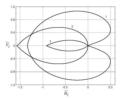
Figure 1: Boundaries of stability region  $S(\alpha)$  for  $\alpha = 0.3$  (boundary 1);  $\alpha = 1$  (boundary 2) and for  $\alpha = 1.6$  (boundary 3).
