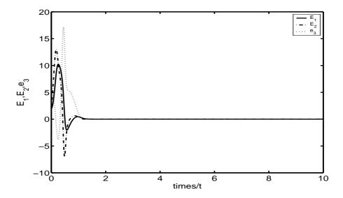
Figure 3. Error dynamics when the controller has been activated, showing that  $(E_1, E_2, e_3)$  are stabilized, implying that the coexistence of synchronization and anti-synchronization in the unified chaotic system is realized.  $\theta = 0$  and  $k_2(0) = -1$ , while the initial conditions are  $x_1(0) = -2, x_2(0) = 3, x_3(0) = 4, y_1(0) = 4, y_2(0) = -1, y_3(0) = -2$ .
