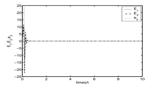
Figure 1. Error dynamics when the controller has been activated, showing that  $(E_1, E_2, e_3)$  are stabilized, implying that the coexistence of synchronization and anti-synchronization in the unified chaotic system is realized.  $\theta = 0.75$  and  $k_1(0) = -1$ , while the initial conditions are  $x_1(0) = -2, x_2(0) = 3, x_3(0) = 4$ ,  $y_1(0) = 4, y_2(0) = -1, y_3(0) = -2$ .
