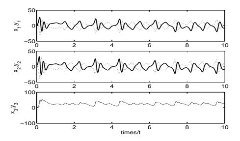
Figure 2. Dynamics of the state variables when controller has been activated.  $x_1, x_2$  anti-synchronizes  $y_1, y_2$  while  $x_3$  synchronizes  $y_3$ .  $\theta = 0.75$  and  $k_1(0) = -1$ , while the initial conditions are  $x_1(0) = -2, x_2(0) = 3, x_3(0) = 4, y_1(0) = 4, y_2(0) = -1, y_3(0) = -2$ .
