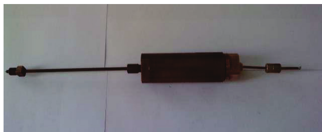
Fig. 6. Photo of high pressure device made from beryllium-bronze alloy used for EPR studies in our laboratory
