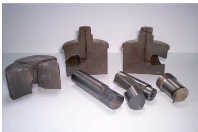
Fig. 14. Elements destroyed by the pressure devices made of bad quality material from a laboratory
