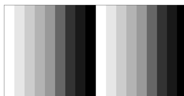
Fig. 2. Image displayed on the monitor while testing parameters of information signals in form of lines in grey level (resolution: 800 × 600, refreshing frequency: 60 Hz)
