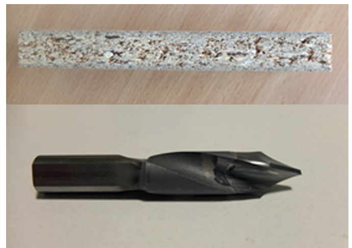
Fig. 1. Standard laminated chipboard and drill used in experiments
