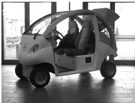
Fig. 12. A two-person version of Elipsa vehicle with a luggage boot
