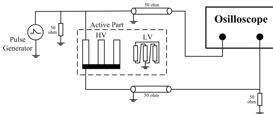
b) Schematic of measurement circuit
