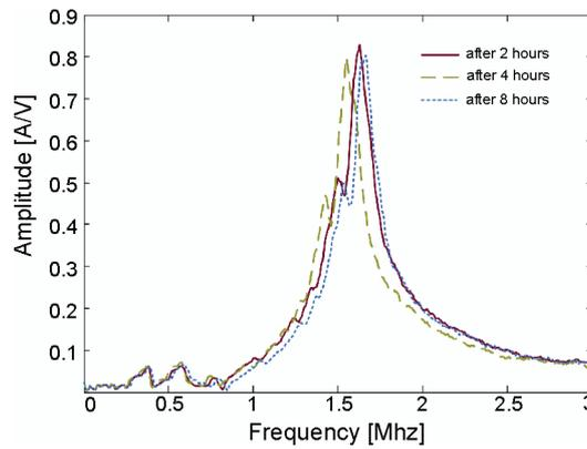
Fig. 2. The measured TFs for three different time intervals (2, 4, and 8 hours) during early hours of process
