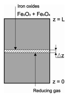
Fig. 3. Model scheme of counter-flow of feedstock and gas
