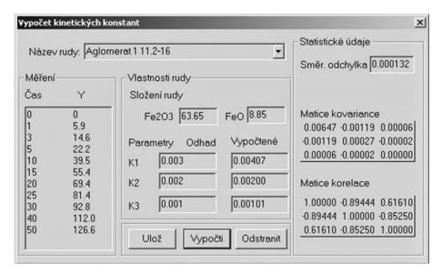
Fig.6. Example of dialog box for calculation of kinetic constants from the reducibility test used in the Czech version of the model
