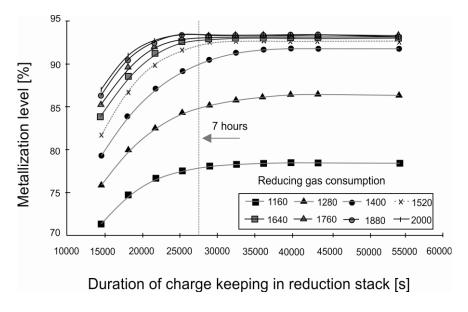
Fig. 8. Reduction course and reducing gas consumption in the stack of reduction aggregate
