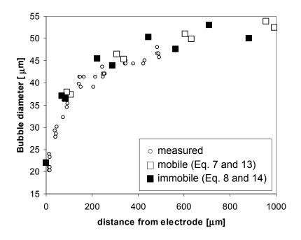
Fig. 7. Calculated and measured bubble diameter ( $D = 190 \,\mu\text{m}$ , current density 152 A/m<sup>2</sup>)
