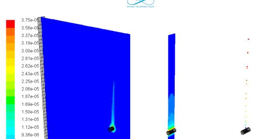
Fig. 4. Hydrogen mass fraction contours at 30 s after current start-up in: (a) x-y, and (b) z-y planes containing the electrode longitudinal (z) axis: (c) shows bubble diameter (scale: 20 (blue) 60 (red) µm) as a function of vertical position (y)
