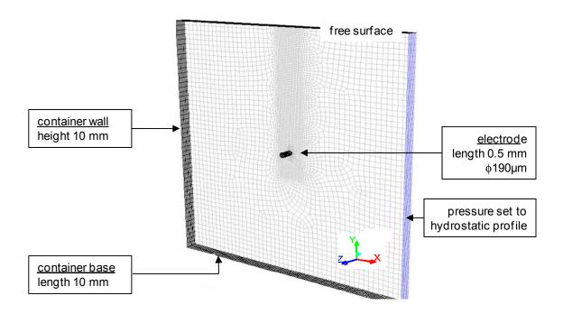
Fig. 2. Geometry and computational mesh
