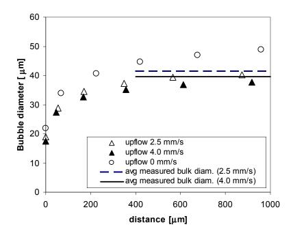
Fig. 9. Effect of liquid upflow on bubble diameter
