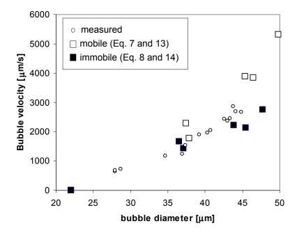
Fig. 8. Calculated and measured velocity of bubbles ( $D = 190 \,\mu\text{m}$ , current density 152 A/m<sup>2</sup>)
