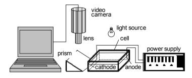
Fig. 1. Experimental apparatus (Sarkar et al., 2010)
