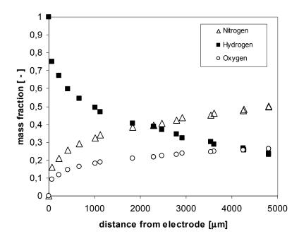
Fig. 10. Composition of gas in bubbles ( $D = 190 \mu \text{m}$ , current density 152 A/m<sup>2</sup>)
