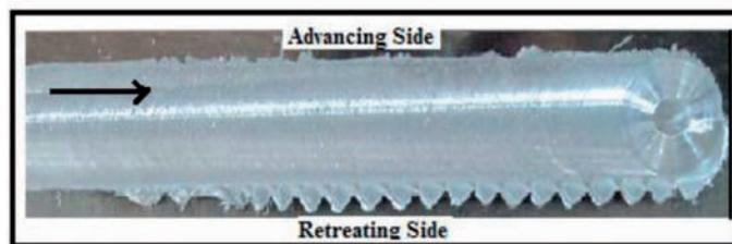
Fig. 8. Advancing and Retreating side of FSW joint of AA6082-T<sub>6</sub>
