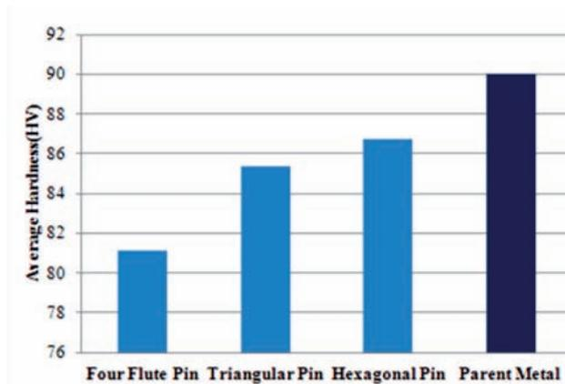
Fig. 7. Average Hardness of AA6082-FSW joint for tool pin profiles
