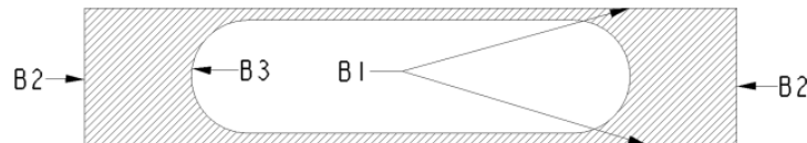
Fig. 2. Gas phase boundary conditions for Eqs. (1)-(2)
