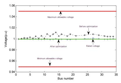
Fig. 10. Voltage profile of 34-buses system before and after optimization
