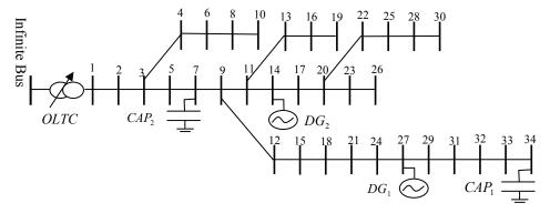
Fig. 8. Single line diagram of 34 buses microgrid
