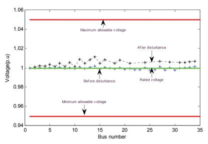
Fig. 9. Voltage profile of 34 buses system before and after disturbance
