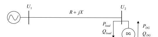
Fig. 1. One-line diagram of a simple two-bus system with DG
