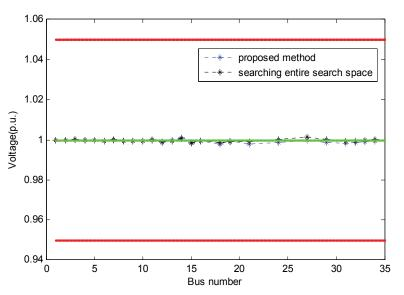
Fig. 12. Comparison of voltage profile of system after optimization by searching the entire search space of control variables method and proposed method
