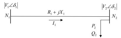
Fig. 2. One-line diagram of a simple two-bus system
